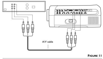
Connecting the projector to a video player using the standard A/V cable
